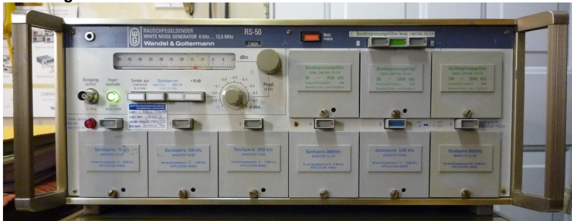
Fig.6: The Wandel & Goltermann RS-50 White Noise Generator.
