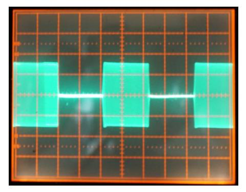
**Test B2b: CW keying sidebands:** The spectrum analyser is coupled to the DUT RF output via the line sampler. The -10 dBm reference level equates to 100W. A series of dits is transmitted at 60 wpm.
