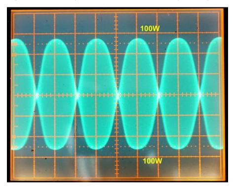
Test B3c: ALC compression tests using white noise: The test instrument (oscilloscope terminated in  $50\Omega$ , then spectrum analyser) is cnnected to the DUT RF output via the power attenuator. The tone/noise generator program in the connected laptop feeds white noise to the DUT USB port.
