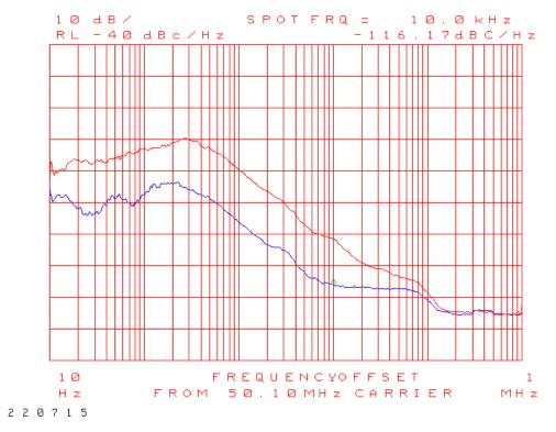
Figure 12c: Transmitted composite noise, 144.1 and 432.1 MHz, 100W.
