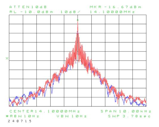
**Test B3: ALC compression tests:** The purpose of these tests is to identify increased transmitter IMD caused by ALC action at high baseband levels, and to check for ALC overshoot (power spikes). *It should be noted here that no overshoot whatsoever was detected.*
