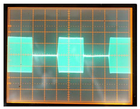
Figure 2: CW keying envelope, 60 wpm, 2ms rise-time, 100W. 10 ms/hor. div.
