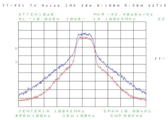
**Test B4: TX IMD test using 2-tone test signal:** The spectrum analyser is connected to the DUT RF output via the power attenuator. The tone/noise generator program in the connected laptop feeds the 2-tone test signal to the DUT USB port. Figures 11a through 11e are the test plots.
