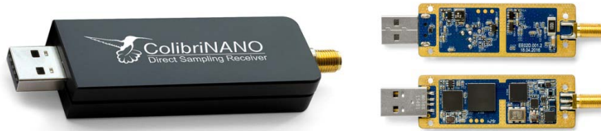
Figure 1: ColibriNANO exterior & interior. (Courtesy Expert Electronics)
