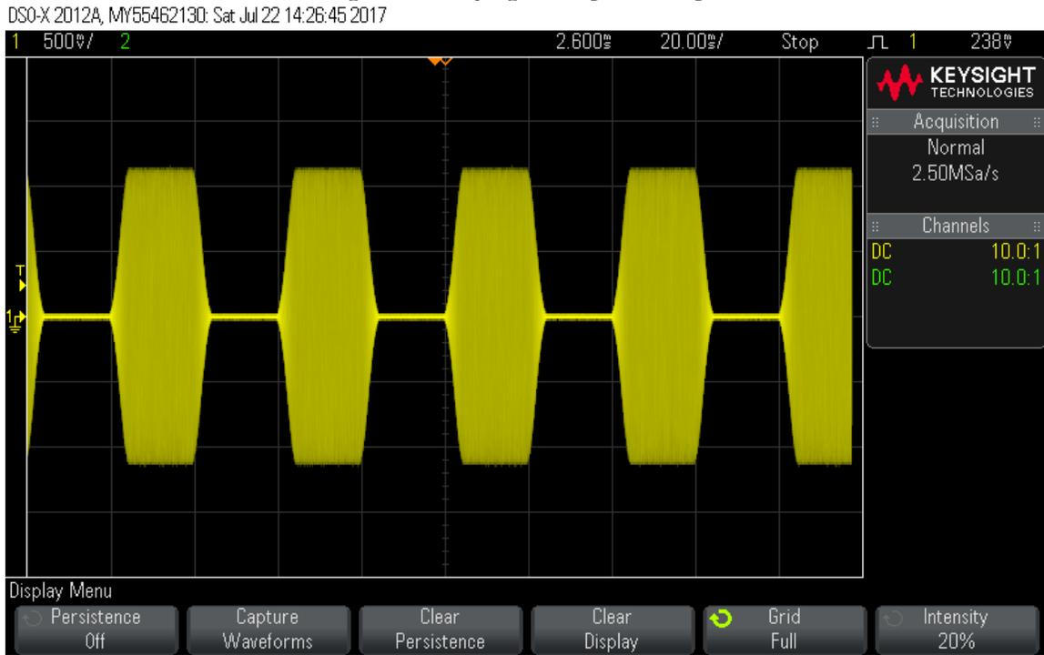
**25: PureSignal Adaptive-Predistortion Linearization Test.**
