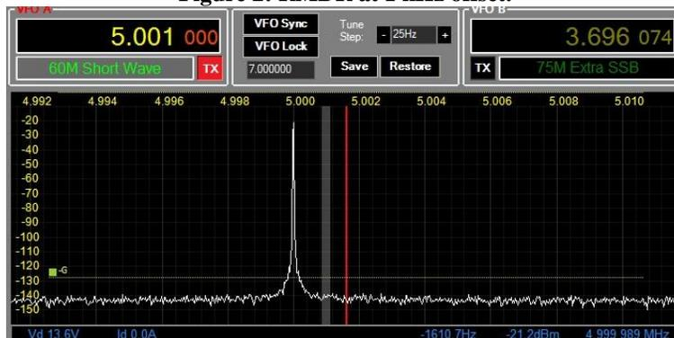
**3: Channel filter shape factor (-6/-60 dB).** This is the ratio of the -60 dB bandwidth to the -6 dB bandwidth, which is a figure of merit for the filter’s adjacent-channel’s rejection. The lower the shape factor, the “tighter” the filter.
