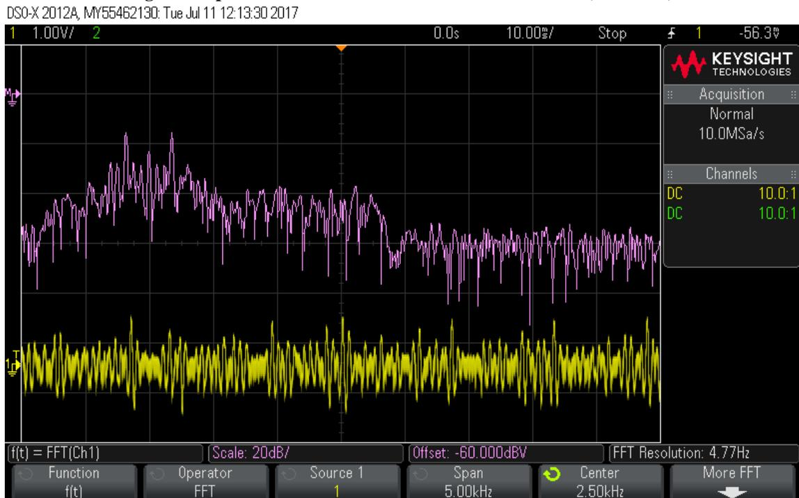
**6: Multi-Notch Filter (MNF) Test.** Since v3.3.6, PowerSDR OpenHPSDR incorporates a new Multi-Notch Filter (MNF) tool, which allows the user to specify up to 1024 notches (bandstop filters). These notches are specified by absolute RF frequency and width; they will be invoked as needed when they overlap the detection passband. This feature is useful for suppressing interference which consistently appears on specific frequencies.
