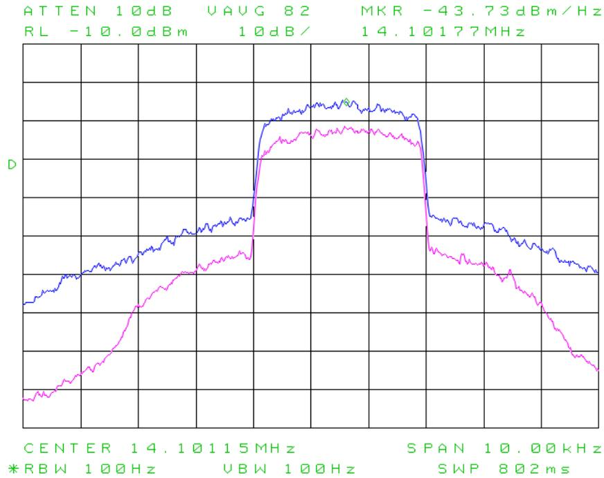
**21: AM sidebands and THD with single-tone modulation.** As in Test 20 above, the spectrum analyzer is connected to the DUT RF output via a 20 dB 25W attenuator. On the GUI, RF Power is adjusted for 50W resting carrier. A 1 kHz test tone is applied from the internal tone generator. The spectrum analyzer records the carrier and sideband parameters.
