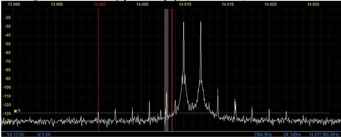
**10: Two-Tone 2<sup>nd</sup>-Order Dynamic Range ( $DR_2$ ).** The purpose of this test is to determine the range of signals far removed from an amateur band which the receiver can tolerate while essentially generating no spurious responses within the amateur band.
