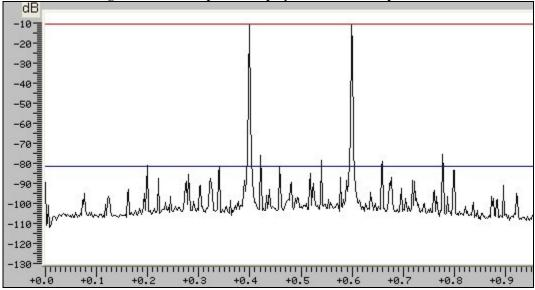
Fig. 12: Baseband spectral display of in-band IMD products.
