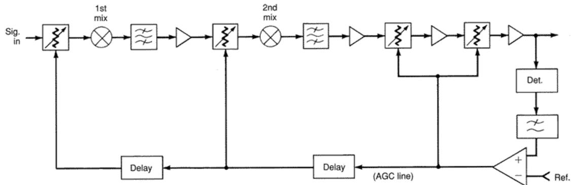
**Figure 4.13** A double-conversion receiver has distributed AGC attenuators to prevent stage overload while also causing the output signal-to-noise ratio to rise with signal increases.
