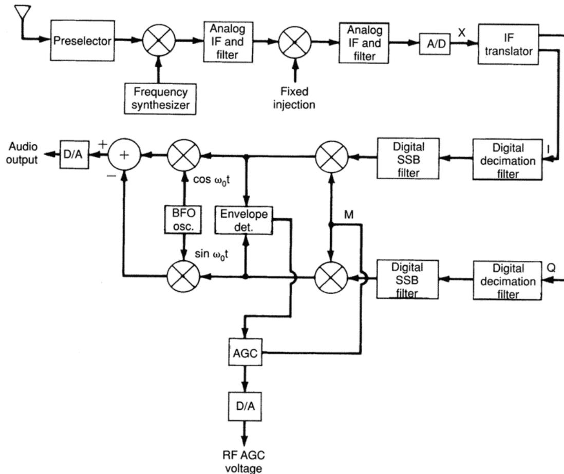
Figure 8.10 Block diagram of a digital SSB receiver.
