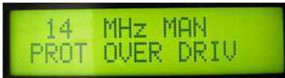
Amplifier has been shut down by the protection circuit and is in a though state.
