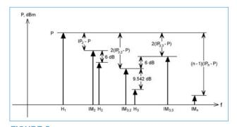
FIGURE 5 Relationship of Harmonics and Intermodulation (IM) Products (5).
